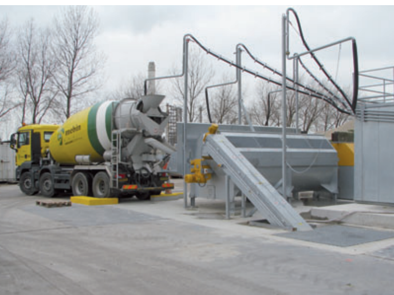
The new Bibko residual concrete recycling system at the Mebin facility in Rotterdam
