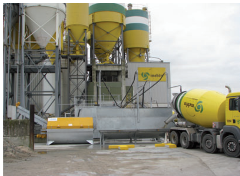
The Bibko residual concrete recycling system in Rotterdam can flush both truck mixers and concrete pumps
